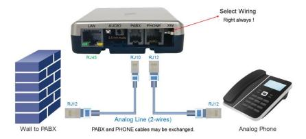
The position of the wire-select switch is always to the right in this case.
