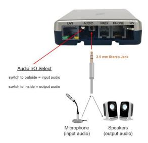
The 3.5 mm stereo audio plug can be set as input or output.
